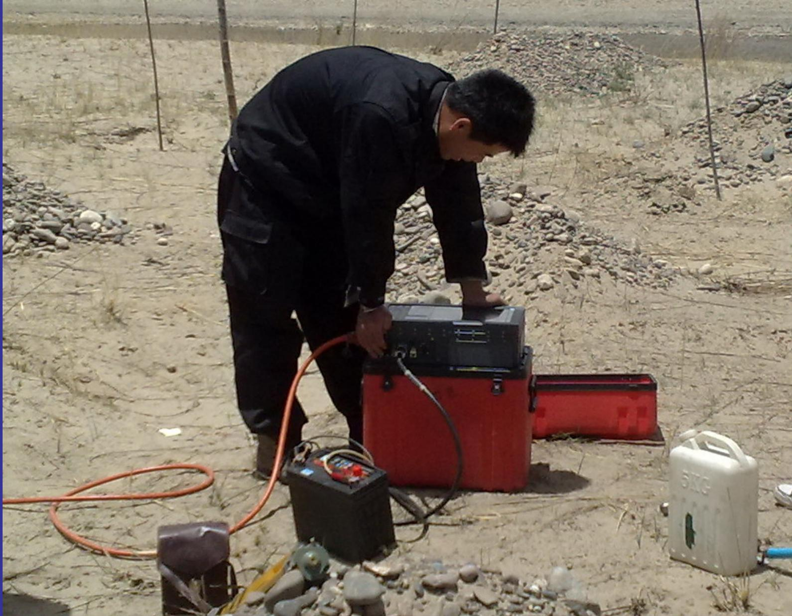
Measuring the depth of deposit with EH4 (Product of GEOMETRICS and EMI)
